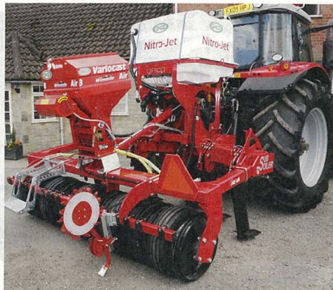
Opico's oilseed rape drilling combination with its subsoiler, fertiliser and seed distribution units, plus the new Synchro roller.
