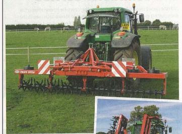
The new Opico hydraulic folding sward slitter is available in 5 and 6m working widths, both have a folded transport width of 2.95m.
